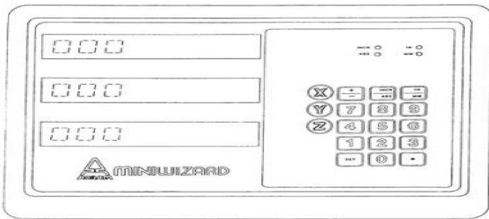
If done properly, all "eights" should appear in each axis display, indicating the start of the diagnostics routine. The routine will then go through various phases of self-check and will end in about 20-30 seconds with a combination of "ones" and "zeros" displayed in each axis.
