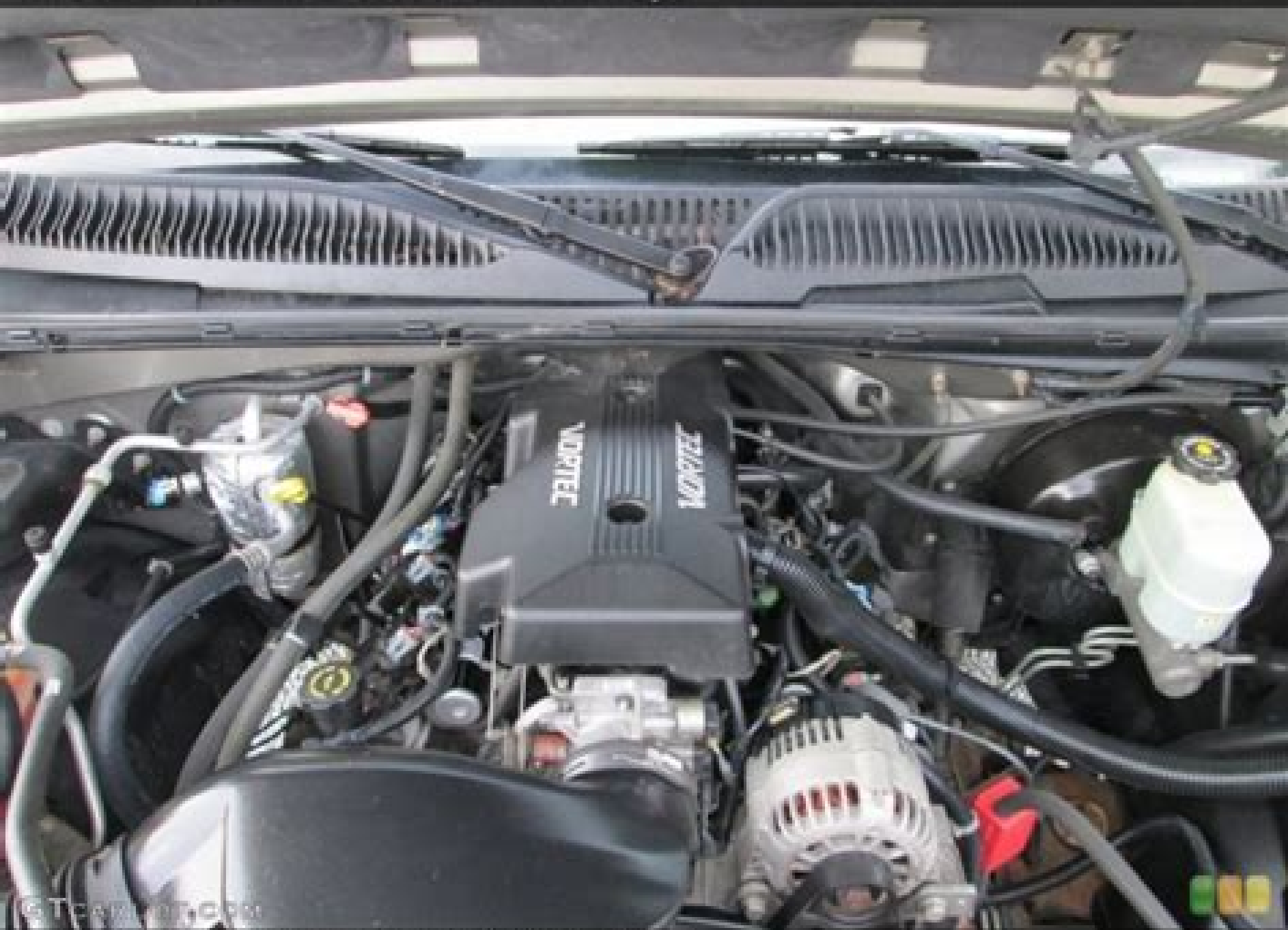
2000 GMC Sierra 1500 SL Extended Cab - 5.3 Liter GMV 16-Valve Vortec V8 Engine
