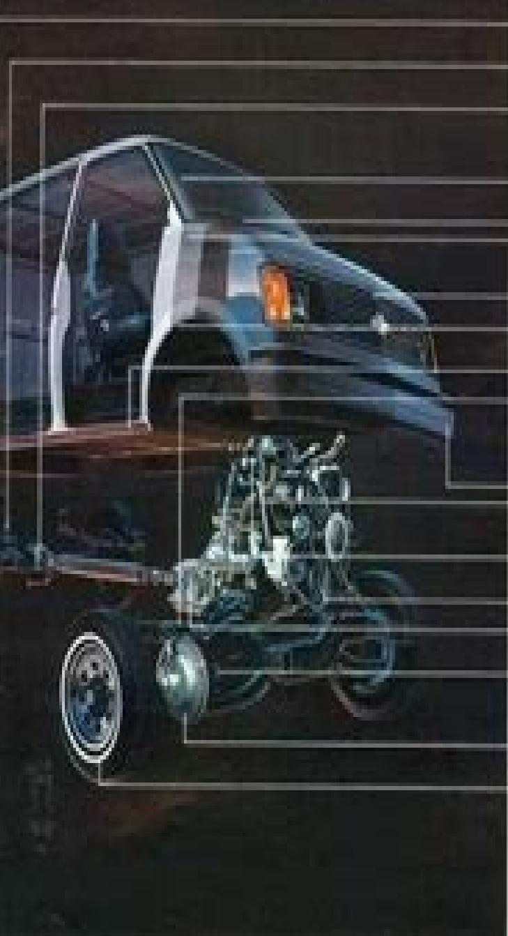
Introducing V-Power. The Vortec V-Power engine is designed to provide improved fuel economy and performance. It is the first Vortec engine to feature a Vortec variable valve timing system.
