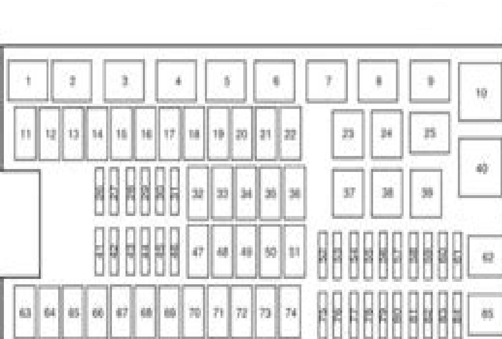
The power distribution box is located in the engine compartment. The power distribution box contains high-current fuses that protect your vehicle's main electrical systems from overloads.
