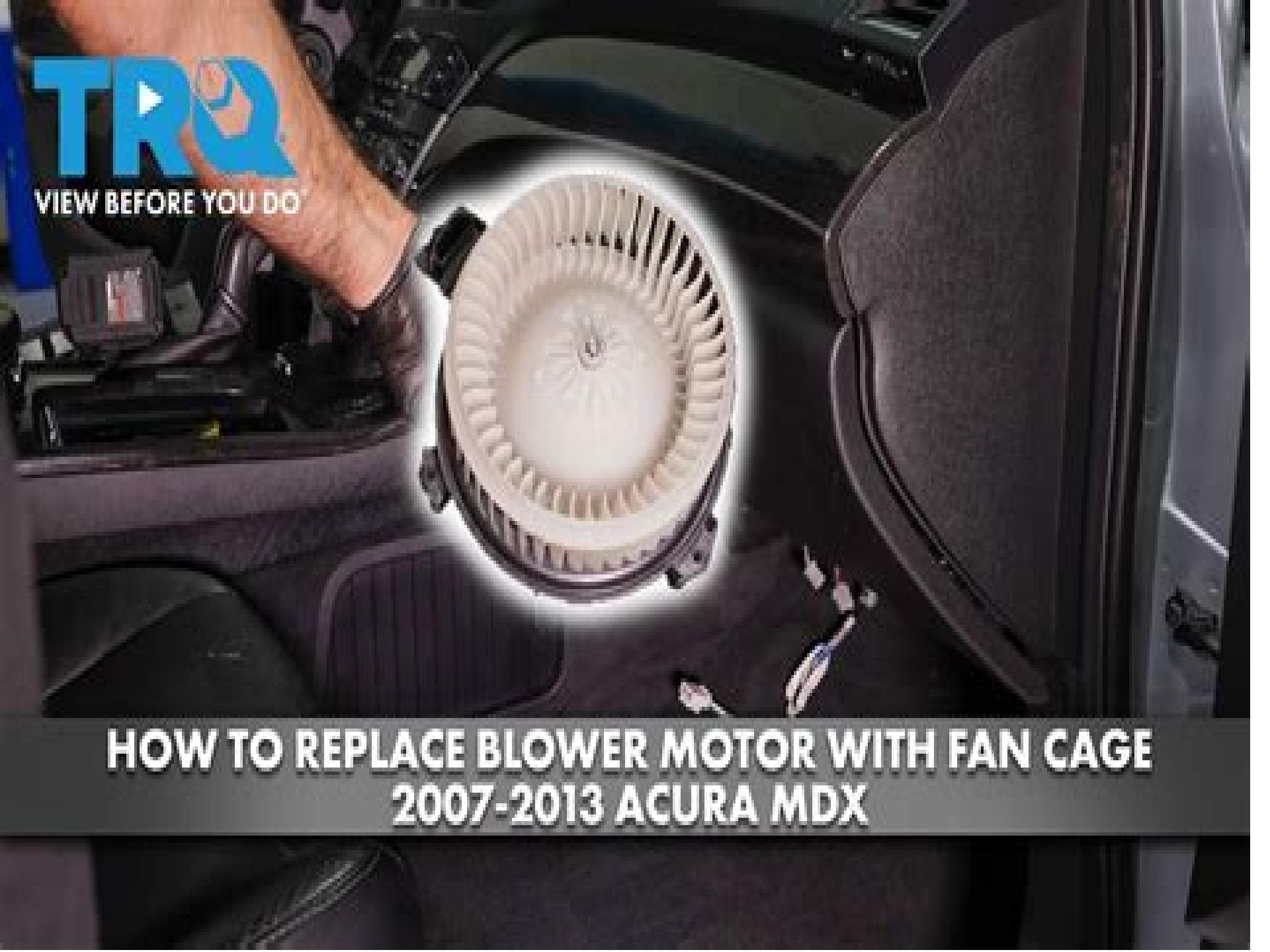
**HOW TO REPLACE BLOWER MOTOR WITH FAN CAGE
