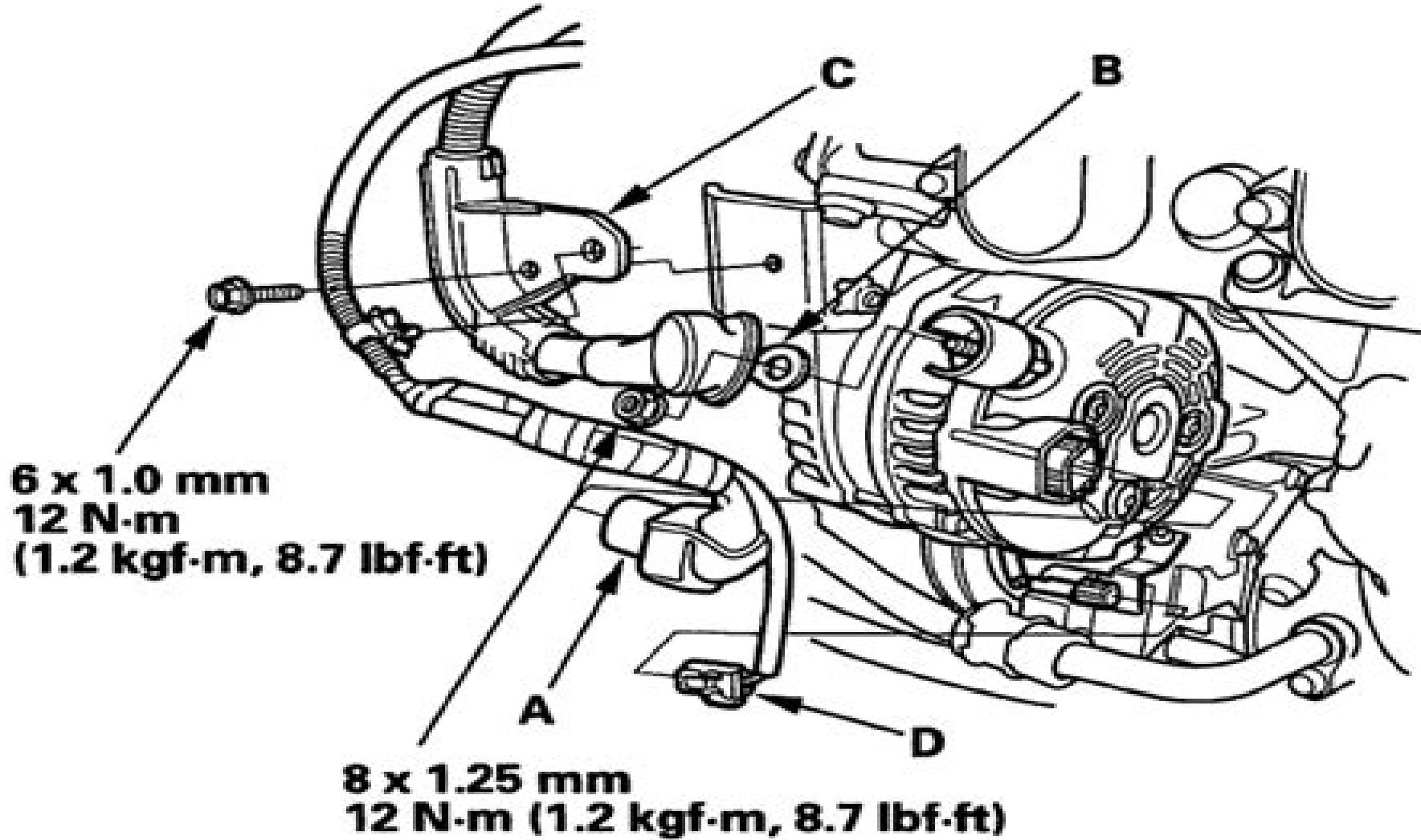
3. Install the harness bracket (C), then connect the A/C compressor clutch connector (D).
