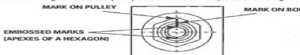
5. Tighten the crank pulley bolt by 60°. (Tighten by one apex of a hexagon of the crank pulley.)
