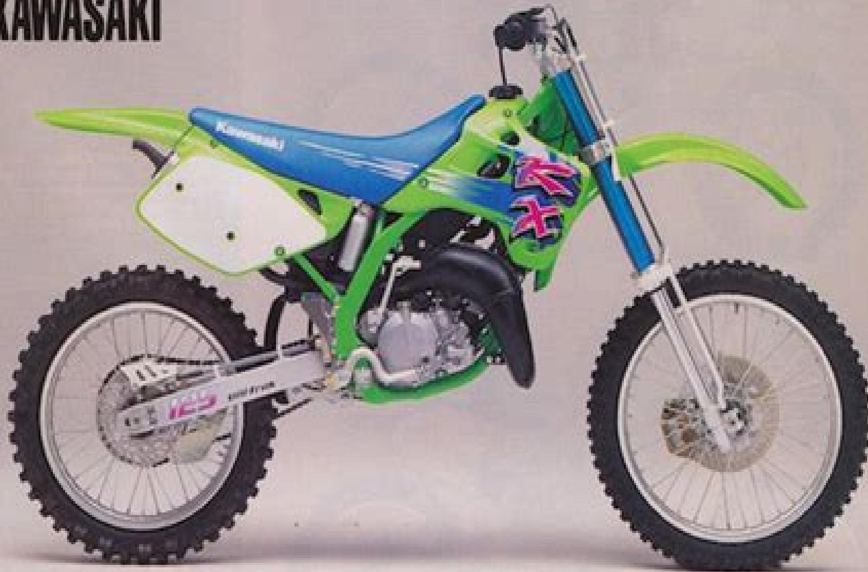
Changes to the KX125 and 250 start with a new frame and plastic. The upper shock mount has been changed (doing away with the bolt-on triangles) and the midsection is slimmer. A lower tank is completely enclosed by the radiator shrouds and the pipe is lower. The silencer is also new. Overall, the bikes look much more sleek, don't you think?
