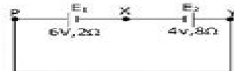
A cell  $E_1$  of EMF 6 volt and internal resistance 2 ohm is connected with another cell  $E_2$  of EMF 4 volt and internal resistance 8 ohm as shown in the figure. Find the potential difference across points X and Y.
