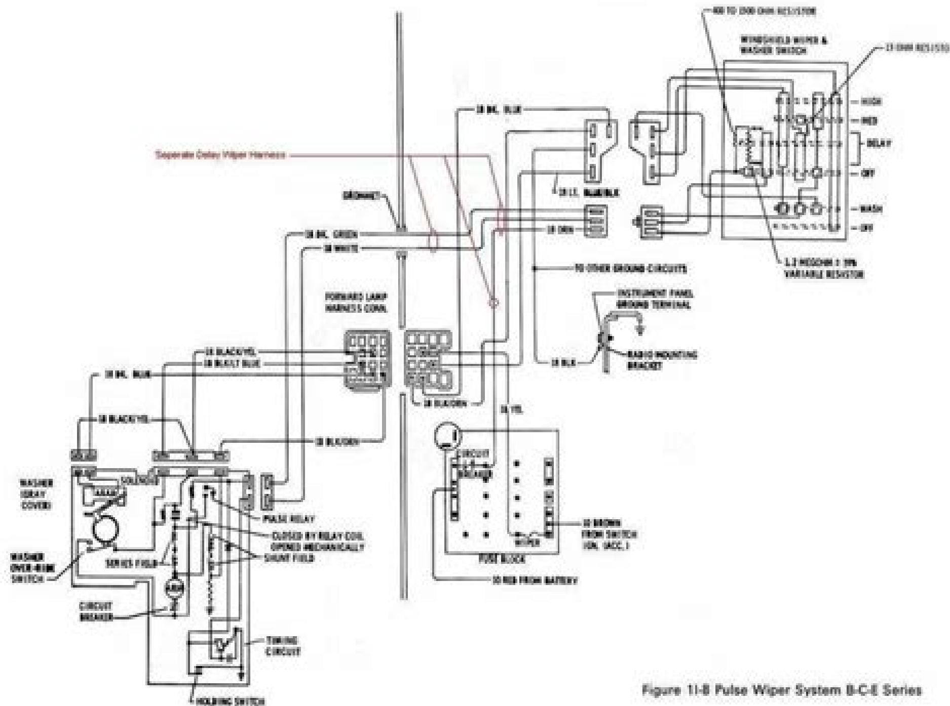
Figure 11-8 Pulse Wiper System B-C4 Series
