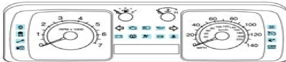
Warning lights and gauges can alert you to a vehicle condition that may become serious enough to cause extensive repairs. A warning light may illuminate when a problem exists with one of your vehicle's functions. Many lights will illuminate when you start your vehicle to make sure the bulbs work. If any light remains on after starting the vehicle, refer to the respective system warning light for additional information.
