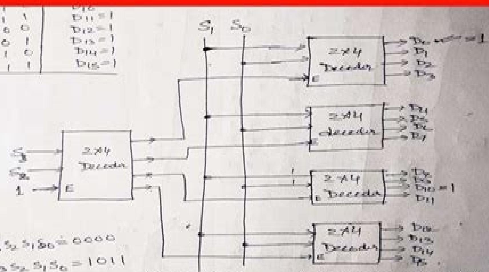
Block diagram of 4x16 decoder using
