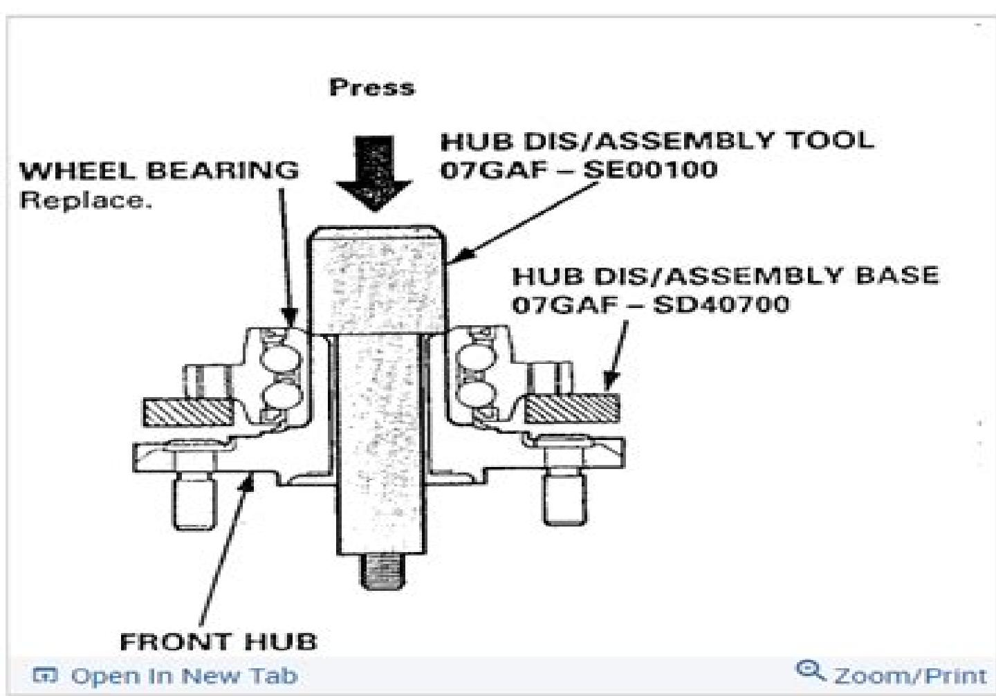
5. Separate the wheel bearing from the front hub using the special tools and a press as shown.
