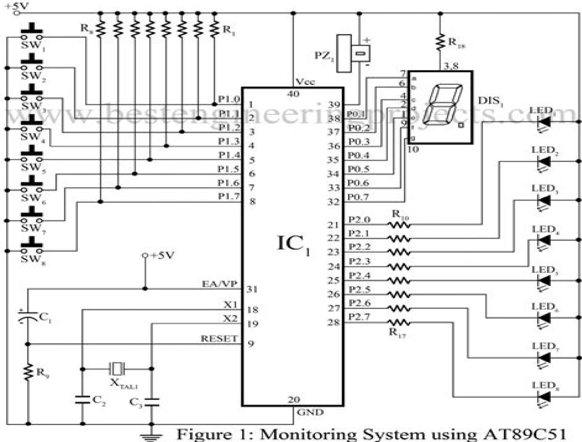
Figure 1: Monitoring System using AT89C51
