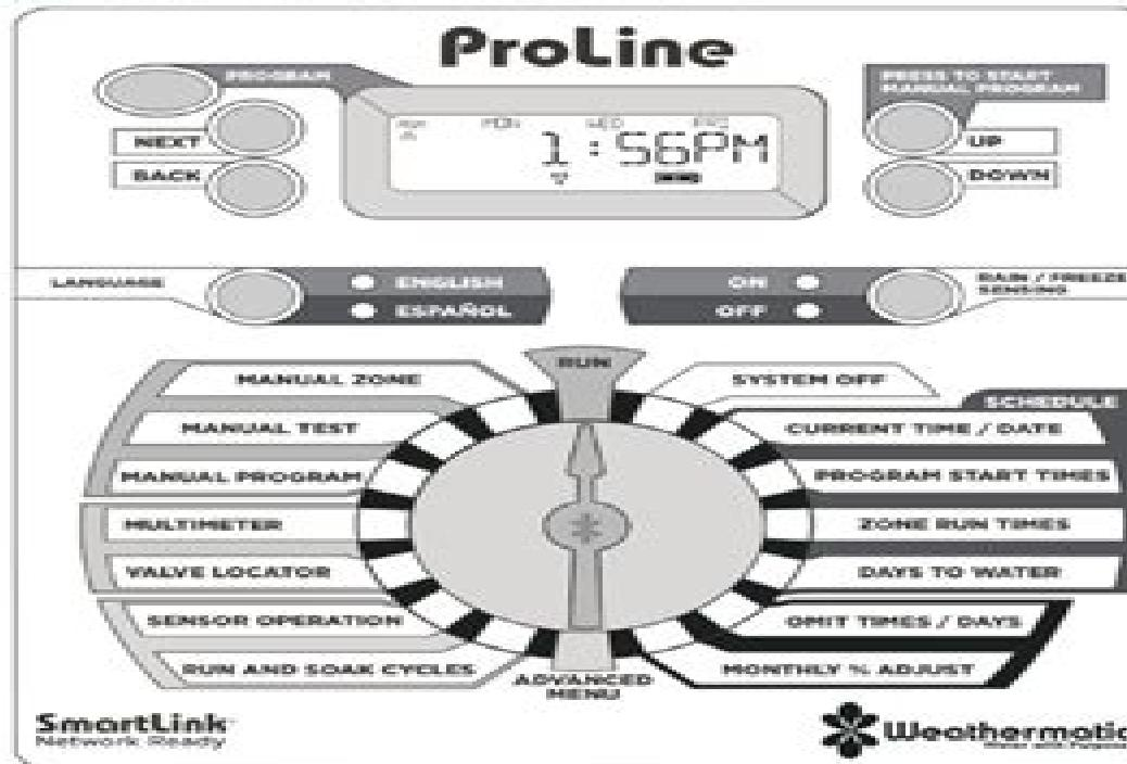
The ProLine® Controller LCD Display provides the following information when the controller is set to RUN, SYSTEM OFF, or when there is no active watering operation underway (display with program in IDLE mode):
