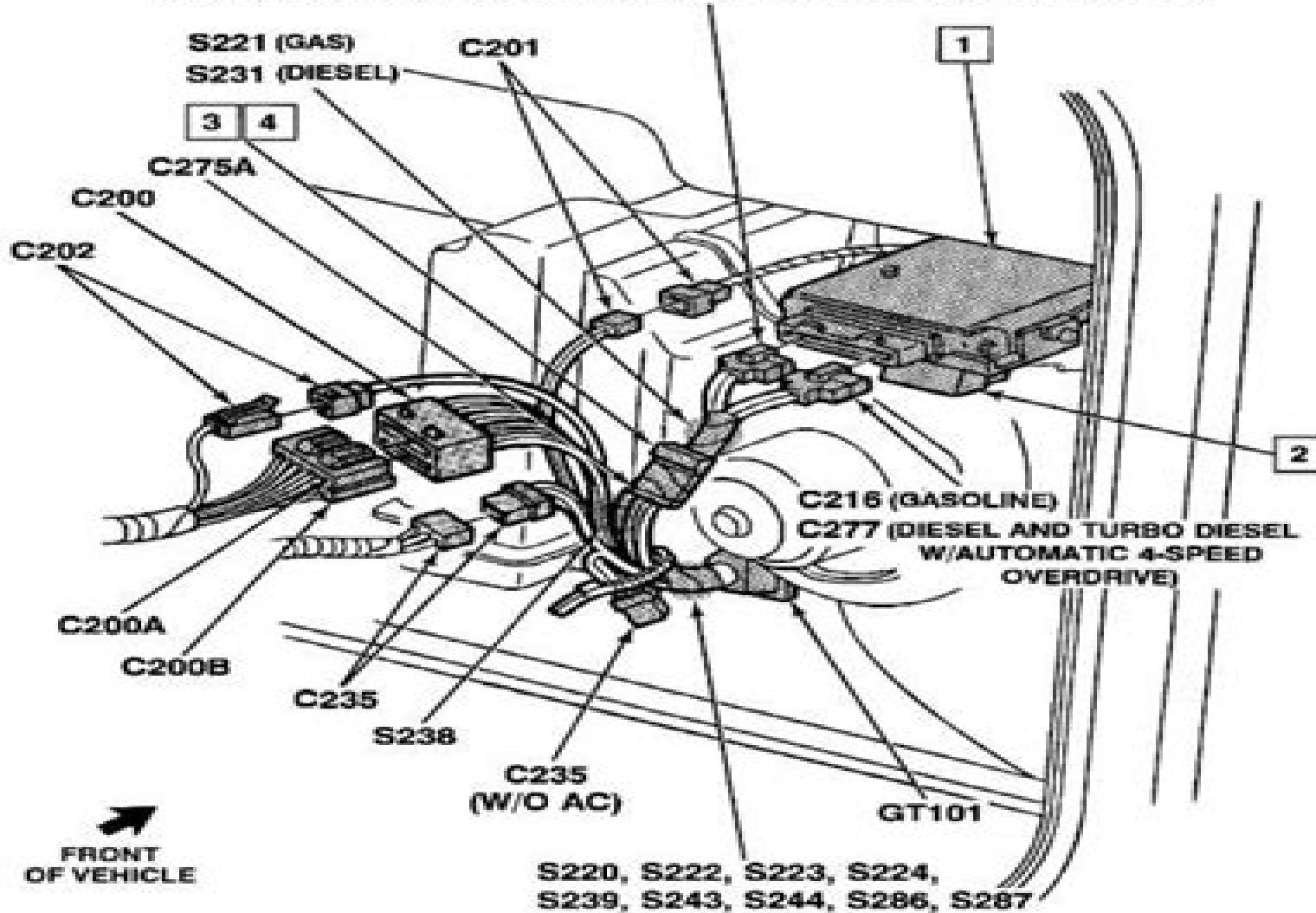
1. ECM - (Gas W/O 4-Speed Automatic Overdrive, W/6.2L Diesel)
