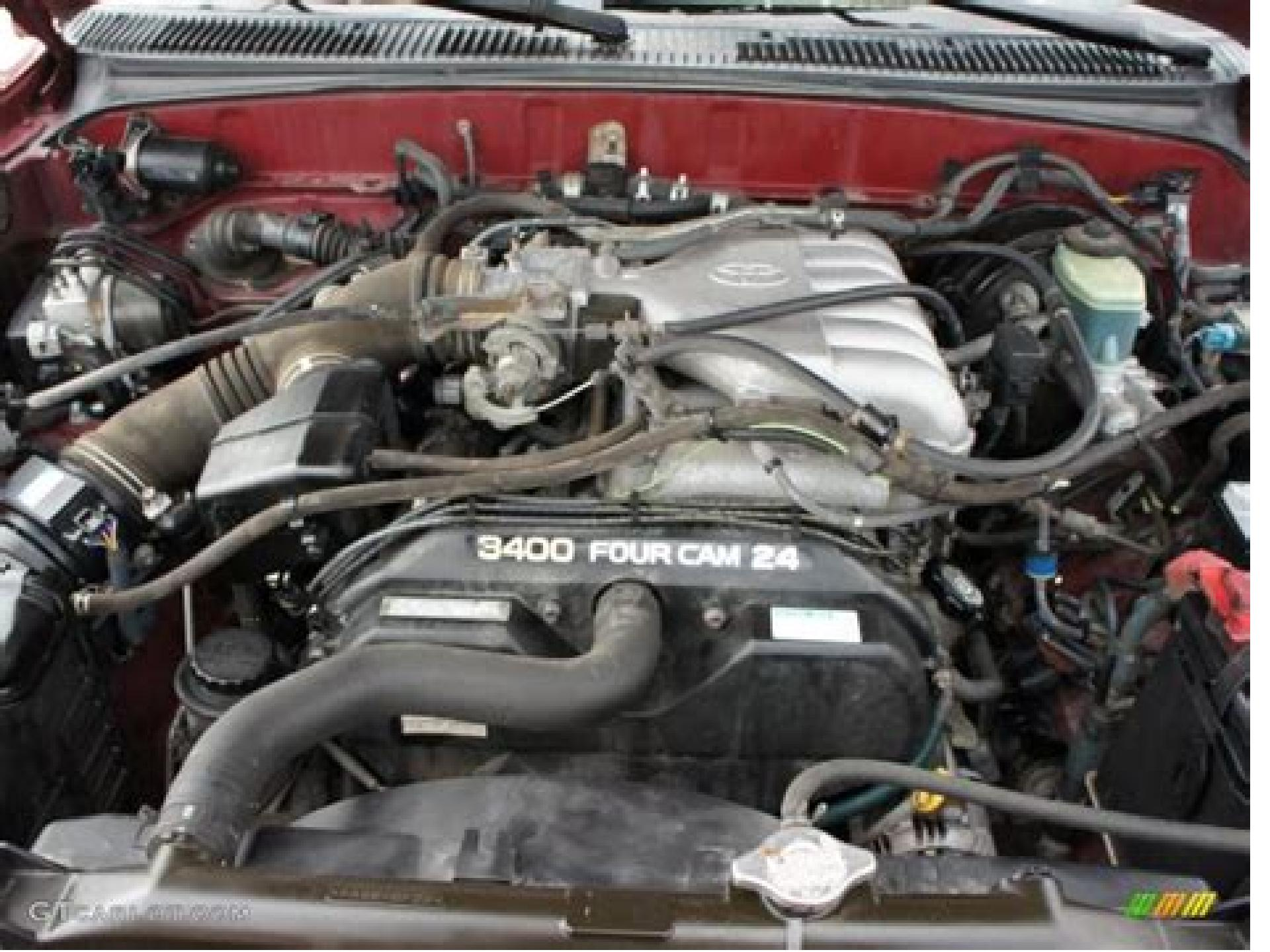
A close-up photograph of a Toyota 3400 Four Cam 24 engine. The engine is a V6 with a red cylinder head. The intake manifold is black with the text "3400 FOUR CAM 24" printed on it. The engine is shown from a front-three-quarter angle, with various hoses, belts, and sensors visible. The Toyota logo is on the cylinder head cover.
