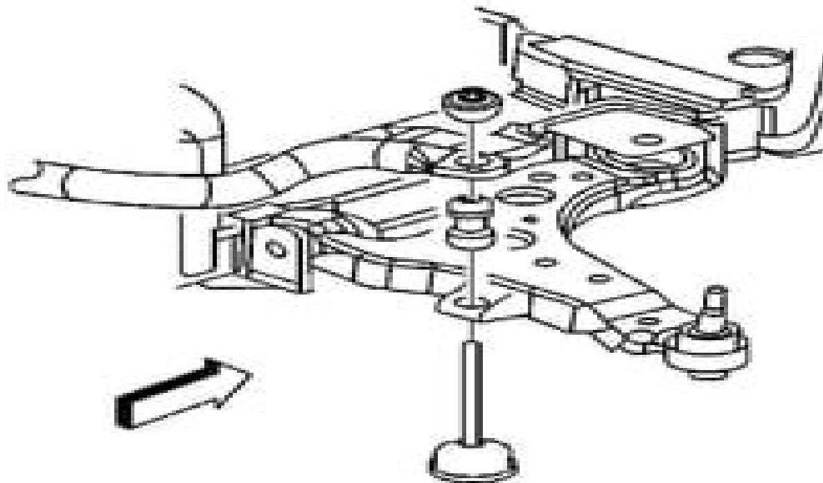
**Fig. 5: View Of Stabilizer Shaft Link Bolt And Nut**
