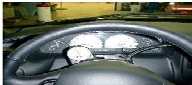
This kit was developed by Ford Racing Performance Parts to allow Ford F150/Harley Davidson or F150 owners the ability to add a vacuum/boost gauge designed to compliment the interior style of the vehicle.
