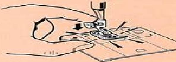
3. Press presser foot screw down firmly until foot snaps into place.
