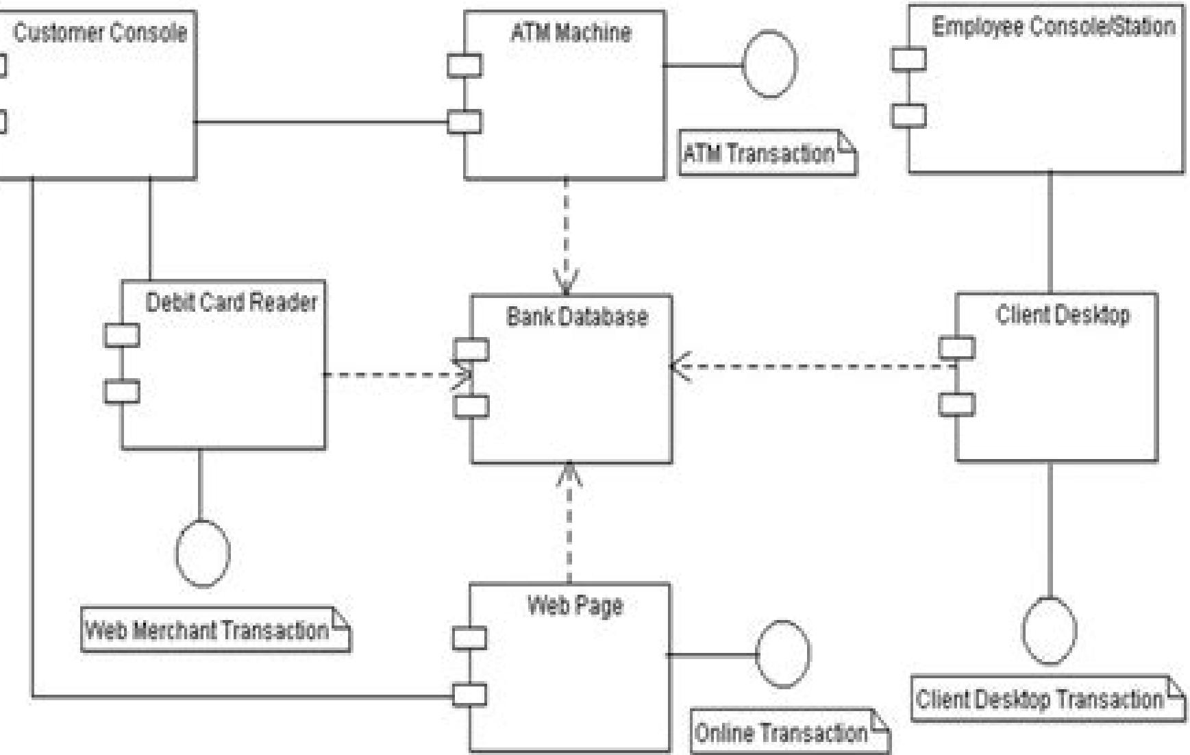
dig.Component diagram of ATM System
