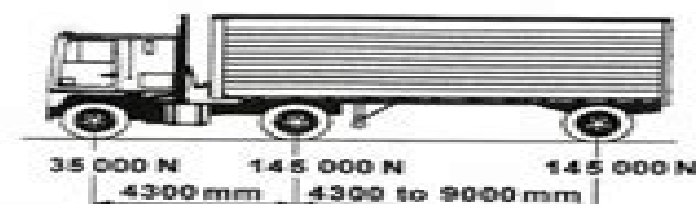
Figure 2(A) Truck loading of HL-93.
