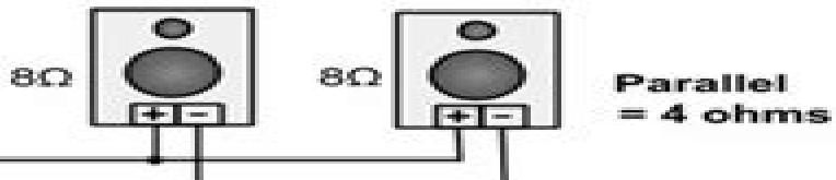
Component speakers (separate tweeter and woofer) are normally wired in parallel and use crossovers for proper sound and to protect the tweeter.
