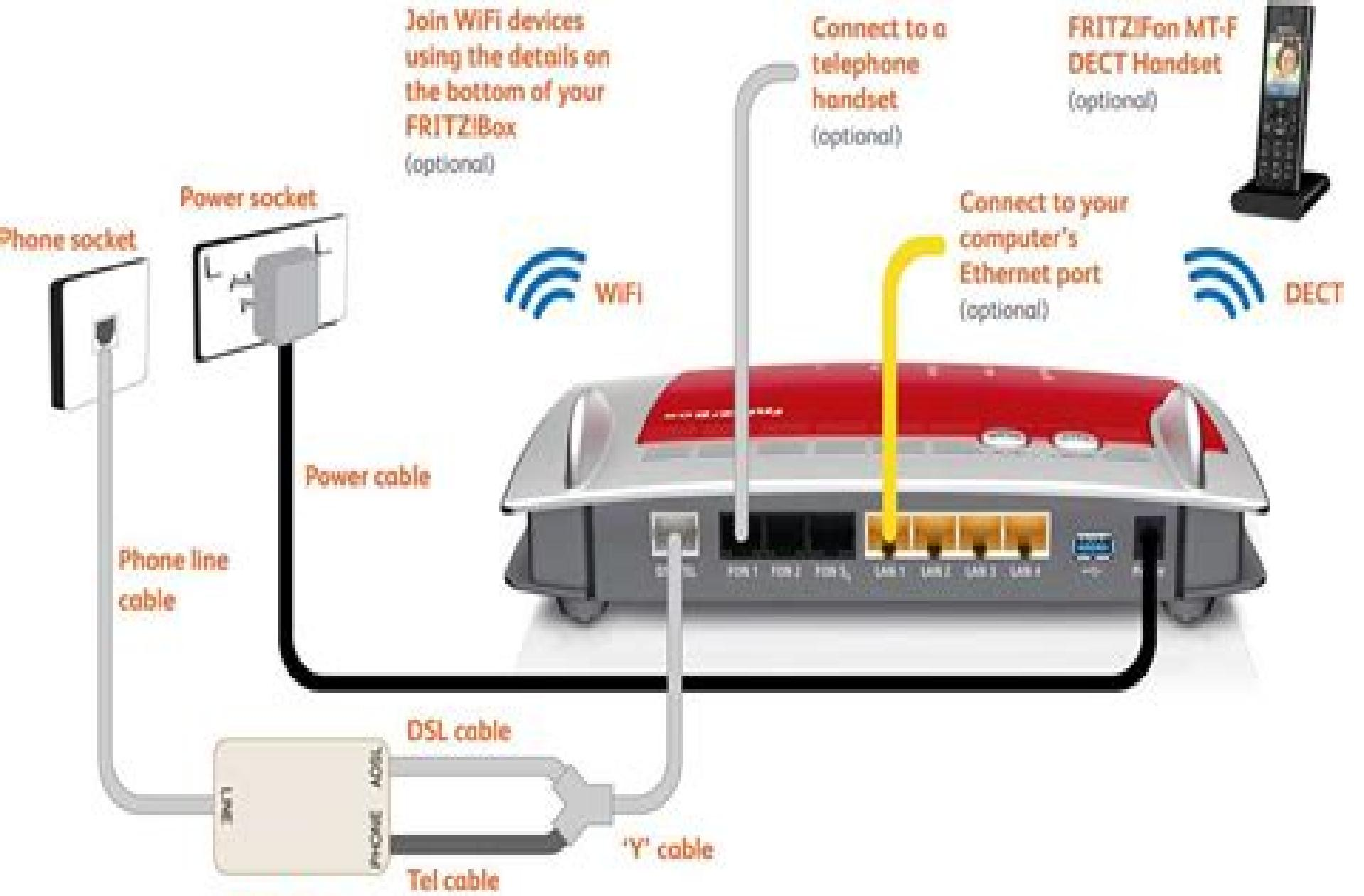
If you have a central splitter wired in to your phone line, with a dedicated wall socket for DSL and your phone, connect the DSL and Tel cables directly to the wall sockets)
