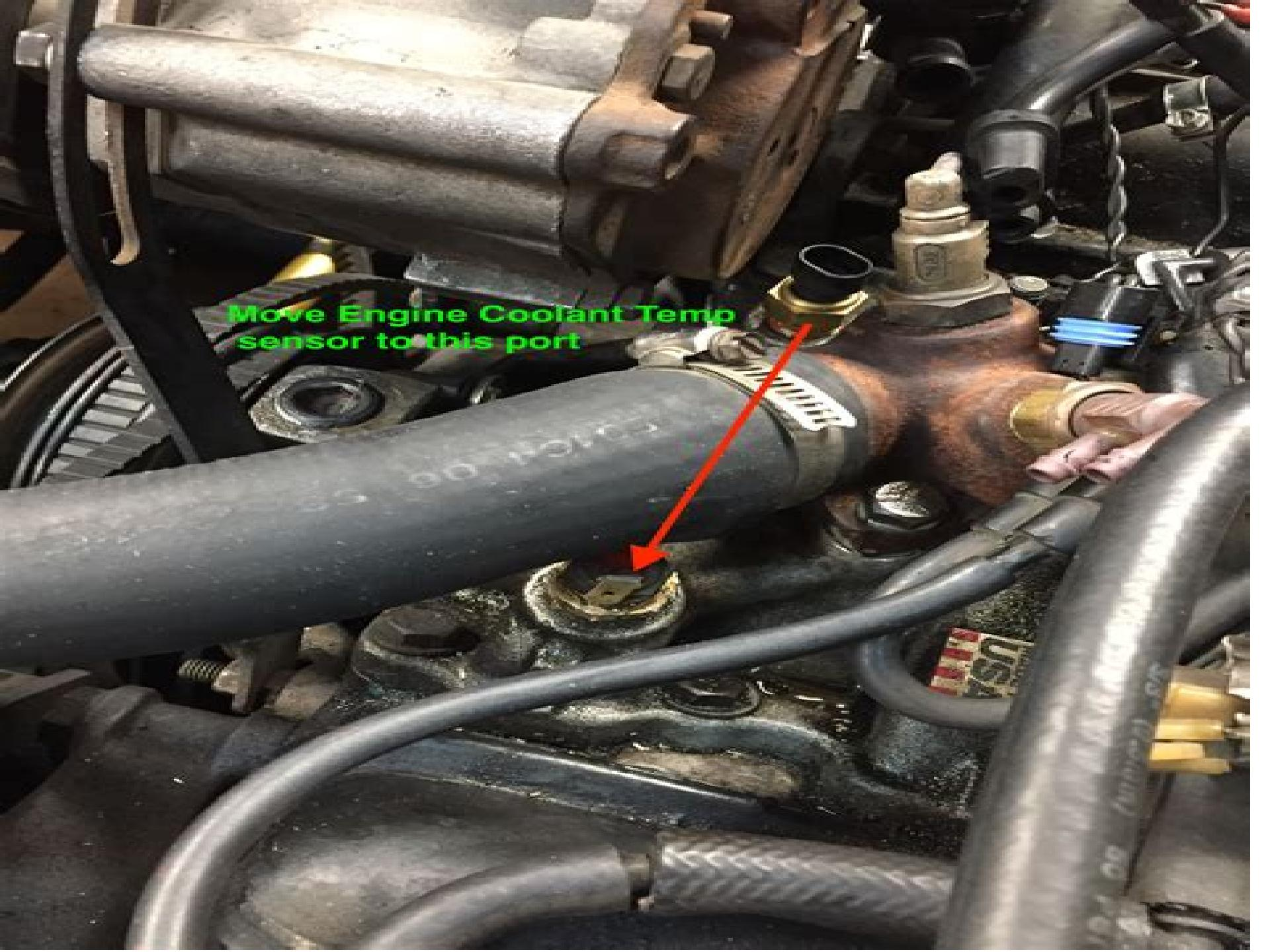
Move Engine Coolant Temp
