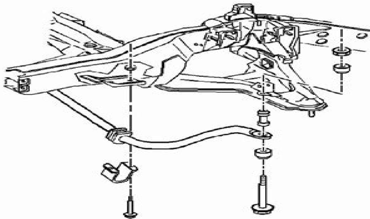
**Fig. 4: View Of Stabilizer Shaft Bracket**
