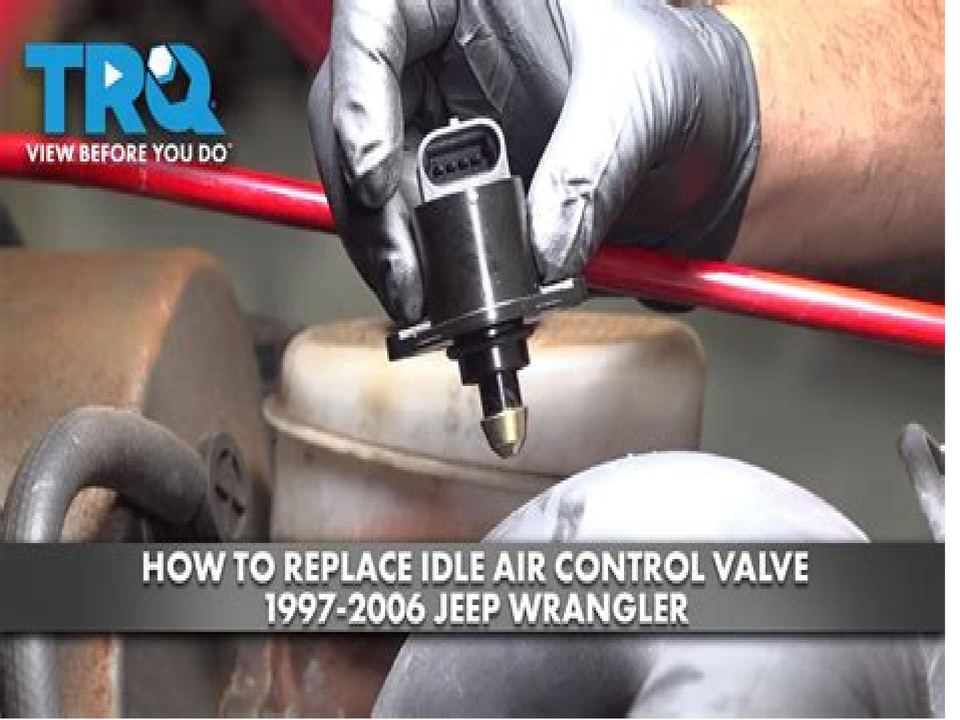
A close-up photograph showing a person's hands wearing black gloves. They are working on the engine of a 1997-2006 Jeep Wrangler, specifically focusing on the idle air control valve. The valve is a black plastic component with a 4-pin electrical connector. A red fuel line is visible in the background. The engine block is a light-colored metal.
