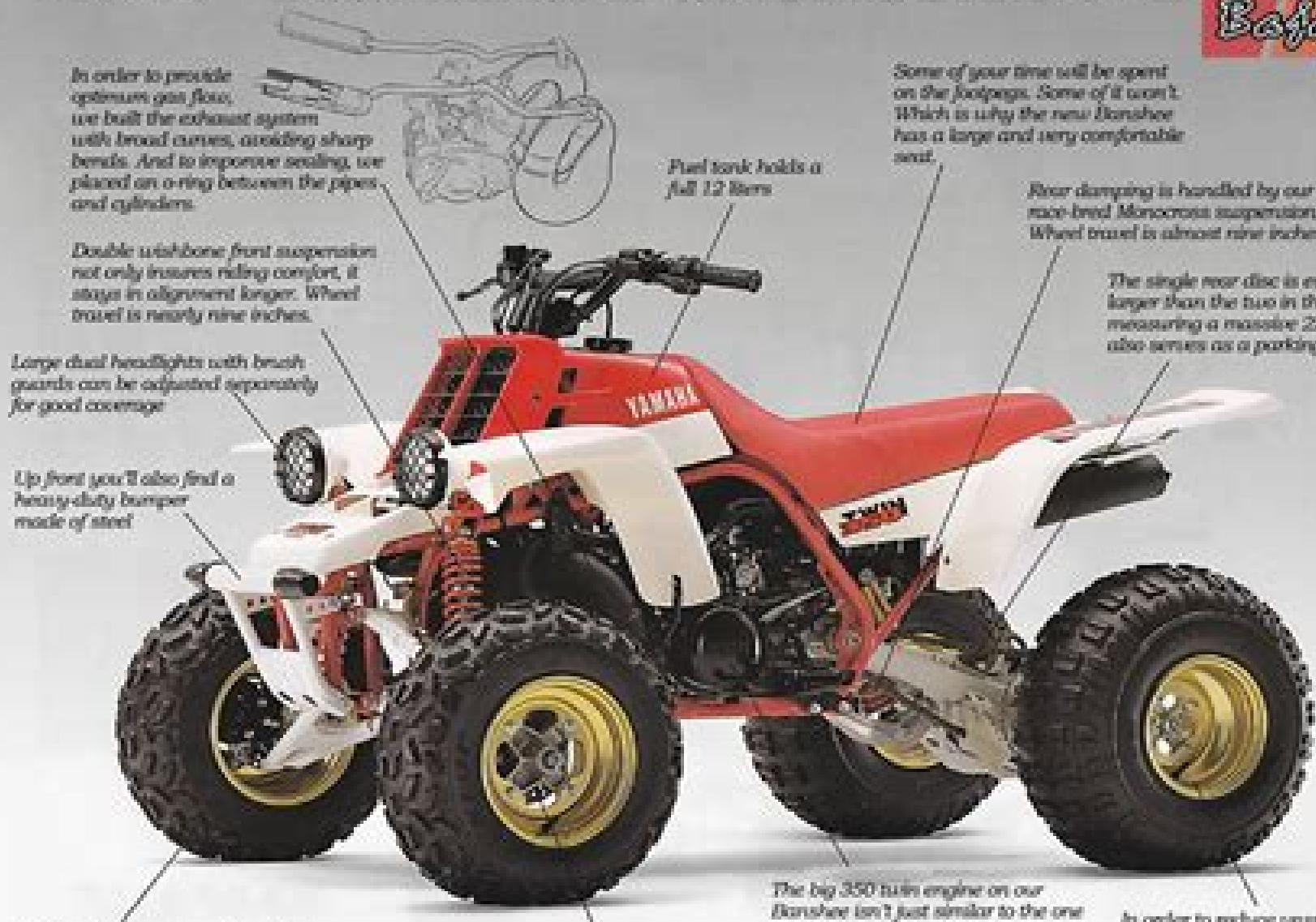
In order to provide optimum gas flow, we built the exhaust system with broad curves, avoiding sharp bends. And to insure sealing, we placed an o-ring between the pipes and cylinders.
