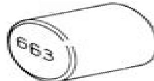
This tool is used for installing the connecting rod small end bearing.
