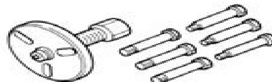
This tool is used for removing the flywheel.
