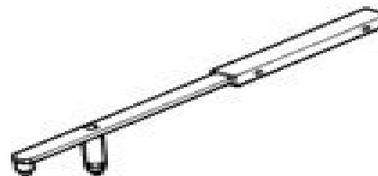
This tool is used for removing and tightening the flywheel securing nut.
