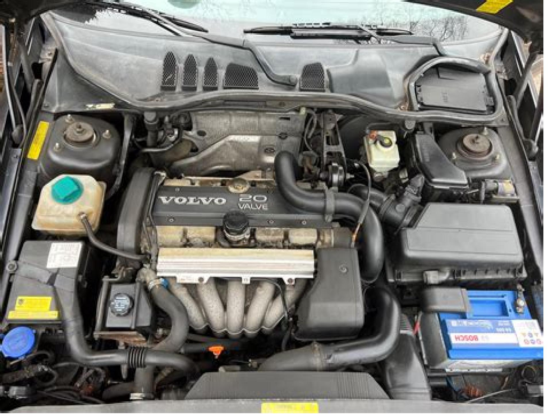
A photograph of the engine compartment of a Volvo car. The engine cover is open, revealing the engine block and various components. The engine block has "VOLVO 20 VALVE" printed on it. The car's body is light blue. The engine cover has a vented top. A white plastic bottle with a green cap is mounted on the left side of the engine. A grey air cleaner box is on the right. A blue Bosch battery is visible at the bottom right. The hood is propped open with a support rod.
