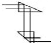
1. The diagram in the above figure shows the prism arrangement in a A. microscope B. stereoscope C. projector D. periscope E. gyroscope
