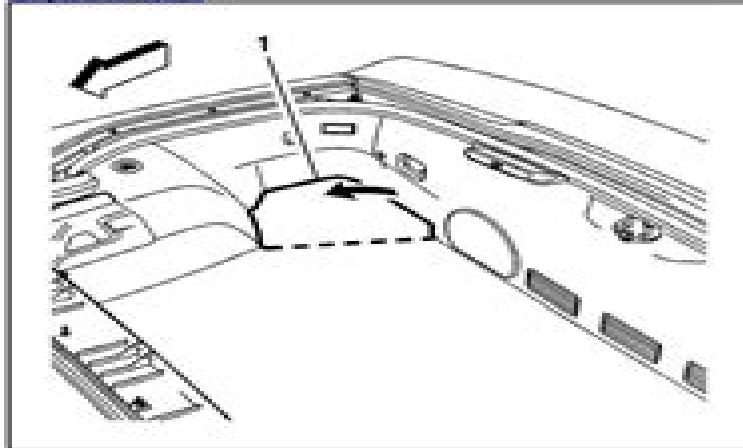
Lift the rear edge of the carpet (1) and fold back along the dotted line, to gain access to the
