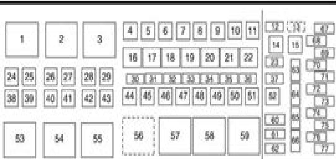
The power distribution box is located in the engine compartment. The power distribution box contains high-current fuses that protect your vehicle's main electrical systems from overloads
