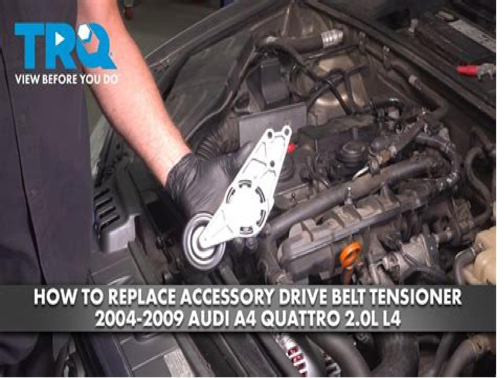
A close-up photograph of the engine compartment of an Audi A4. A person's arm is visible, reaching into the engine bay to remove a white plastic cover from a belt tensioner. The engine block and various hoses and components are visible in the background.
