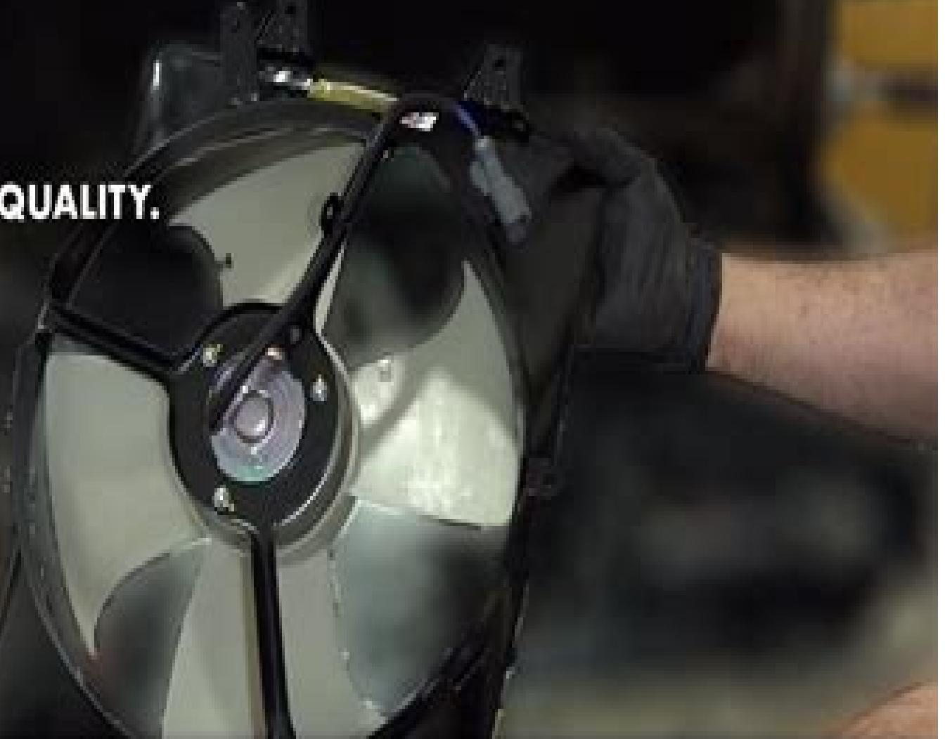
**HOW TO REPLACE AC CONDENSER COOLING FAN ASSEMBLY
