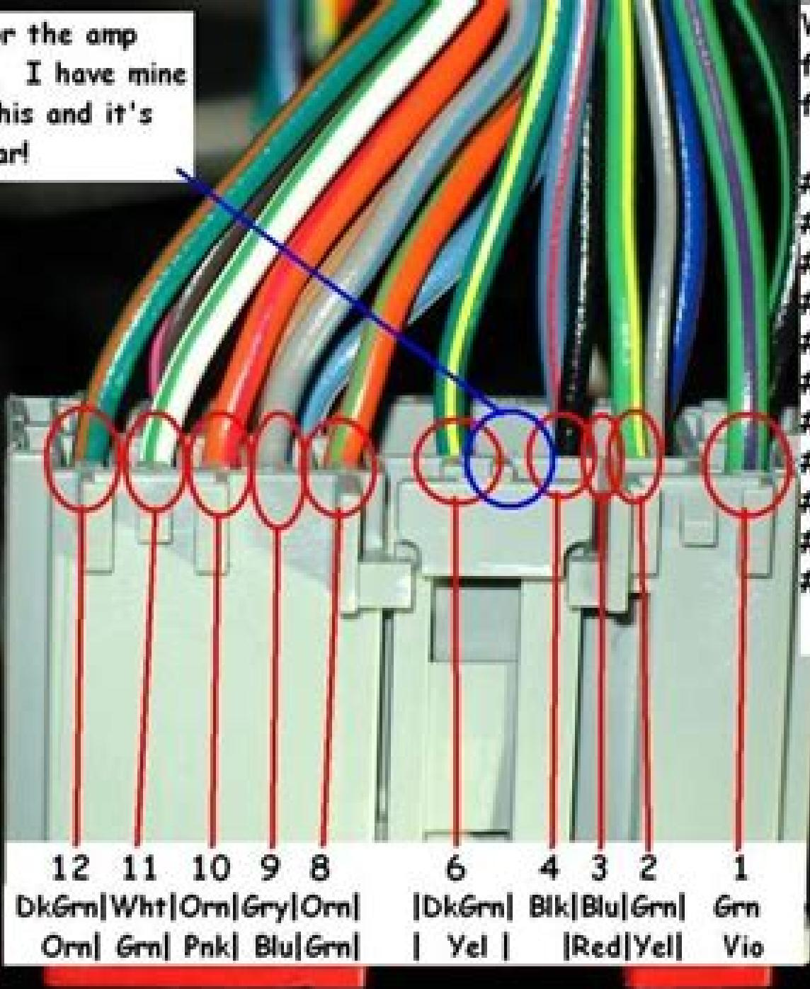
Wiring harness removed from the rear of the factory radio.
