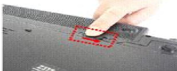
2. Slide the battery latch 2 and pull the whole battery out.
