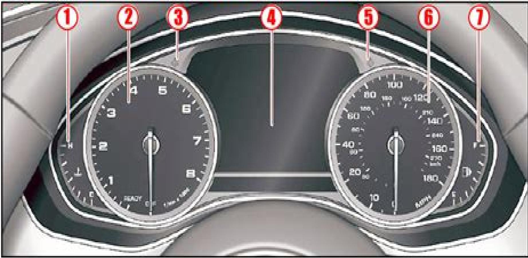
1. Engine Coolant Temperature Gauge;
