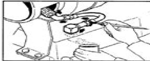
5. Use soap suds or leak detector solution to check hoses, connections and assemblies while system pressure is not less than 90 psi (620 kPa). When hose assemblies with reusable fittings are used, also test between the fitting female and the hose.
