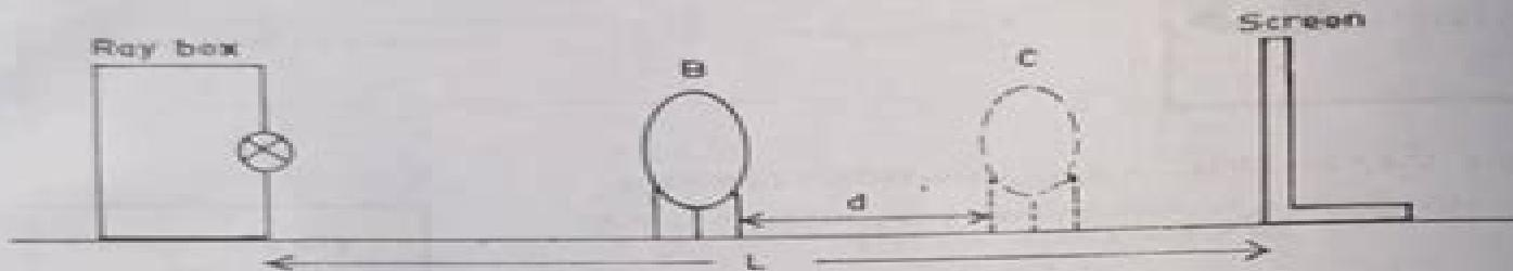
(a) You are provided with a converging lens, ray box, metre rule and other necessary apparatus.
