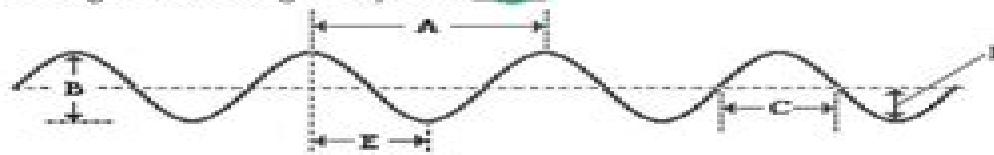
3. A sine curve that represents a transverse wave is drawn below. Use the centimeter ruler to measure the wavelength and amplitude of the wave (show units).
