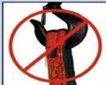
DO NOT place the sling tag in the hook, shackle or connection hardware.
