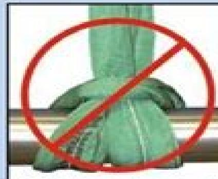
DO NOT allow the sling to roll over itself and twist at the bite of the choker hitch.
