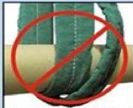
When rigging a basket hitch, DO NOT pull slack out of the hitch with the crane.
