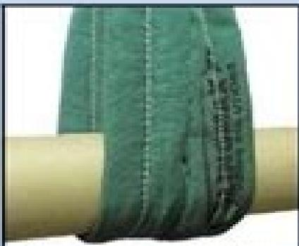
Sling users must take the slack out, before lifting.
