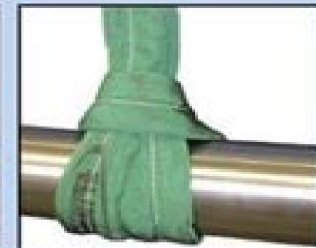
Make sure the paths of the sling run smooth in the bite of the choker hitch without twisting.
