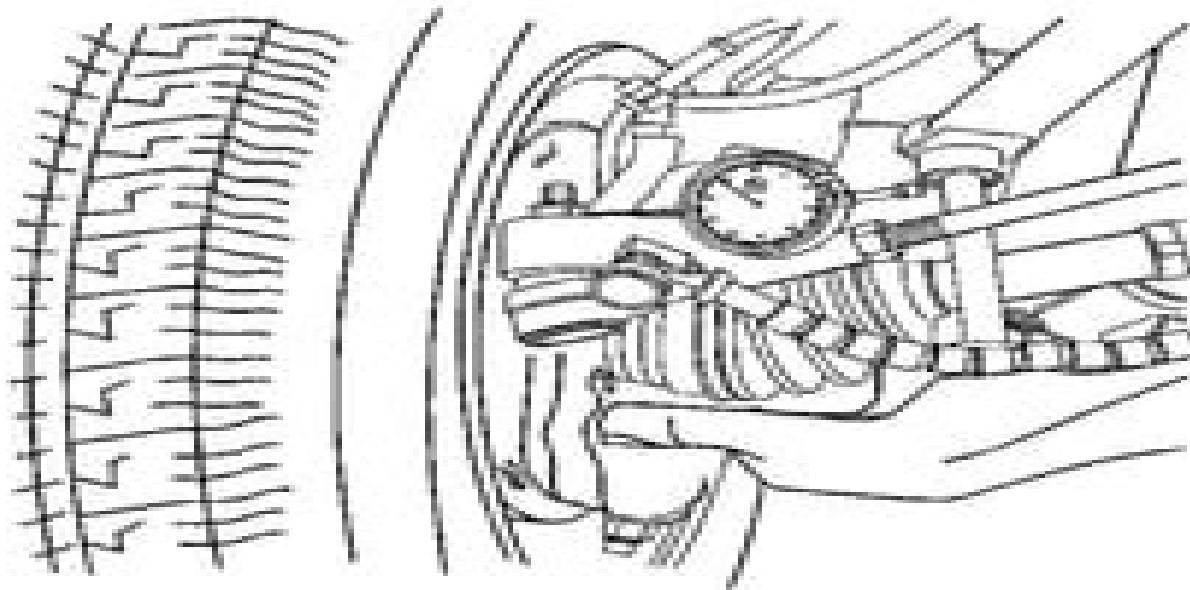
Fig. 7: Installing A Dial Indicator Between The Outer Tie Rod And Steering Knuckle.
