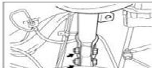
(b) Loosen the 2 nuts on the lower part.
