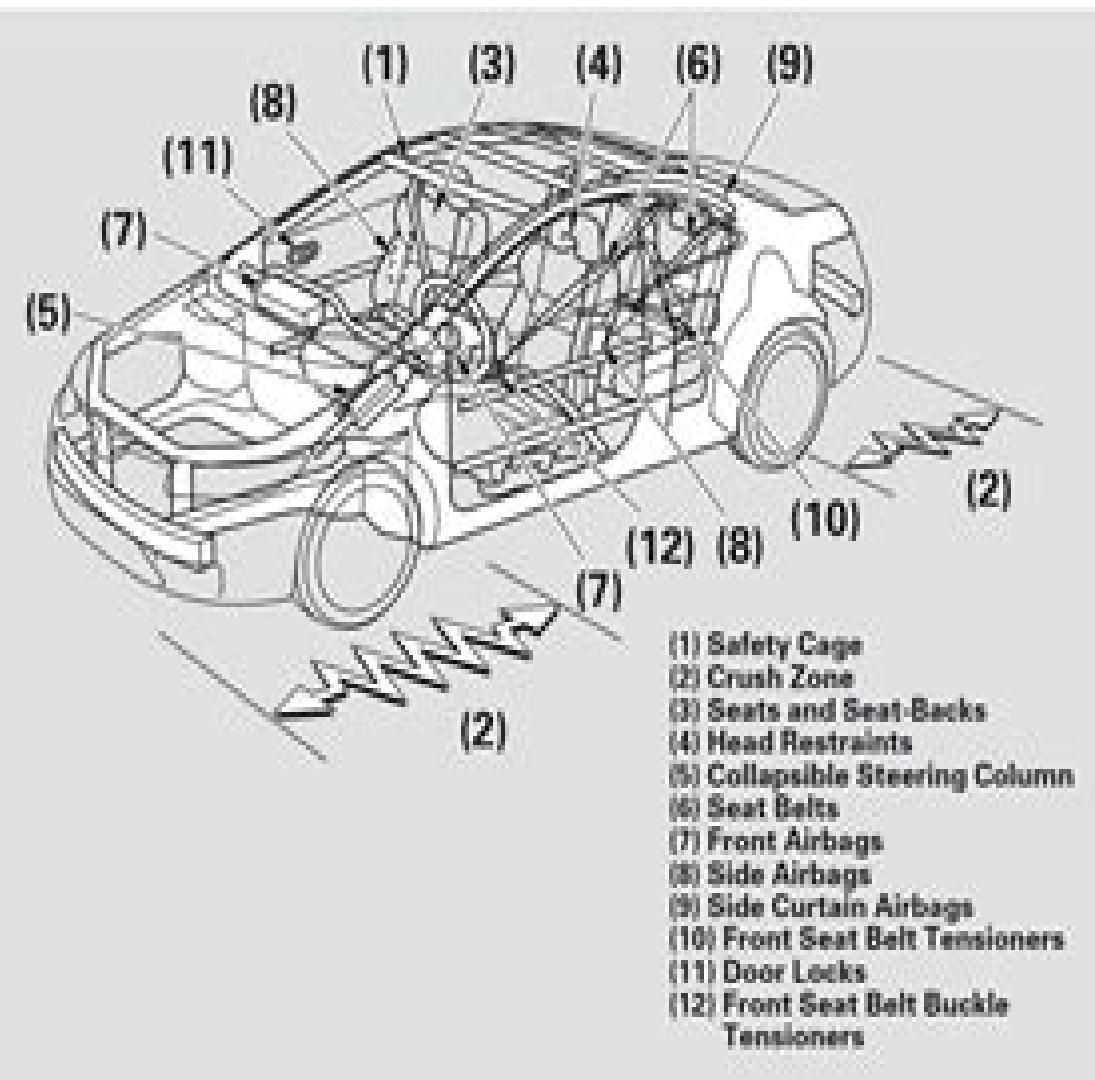
Your vehicle is equipped with many features that work together to protect you and your passengers during a crash.
