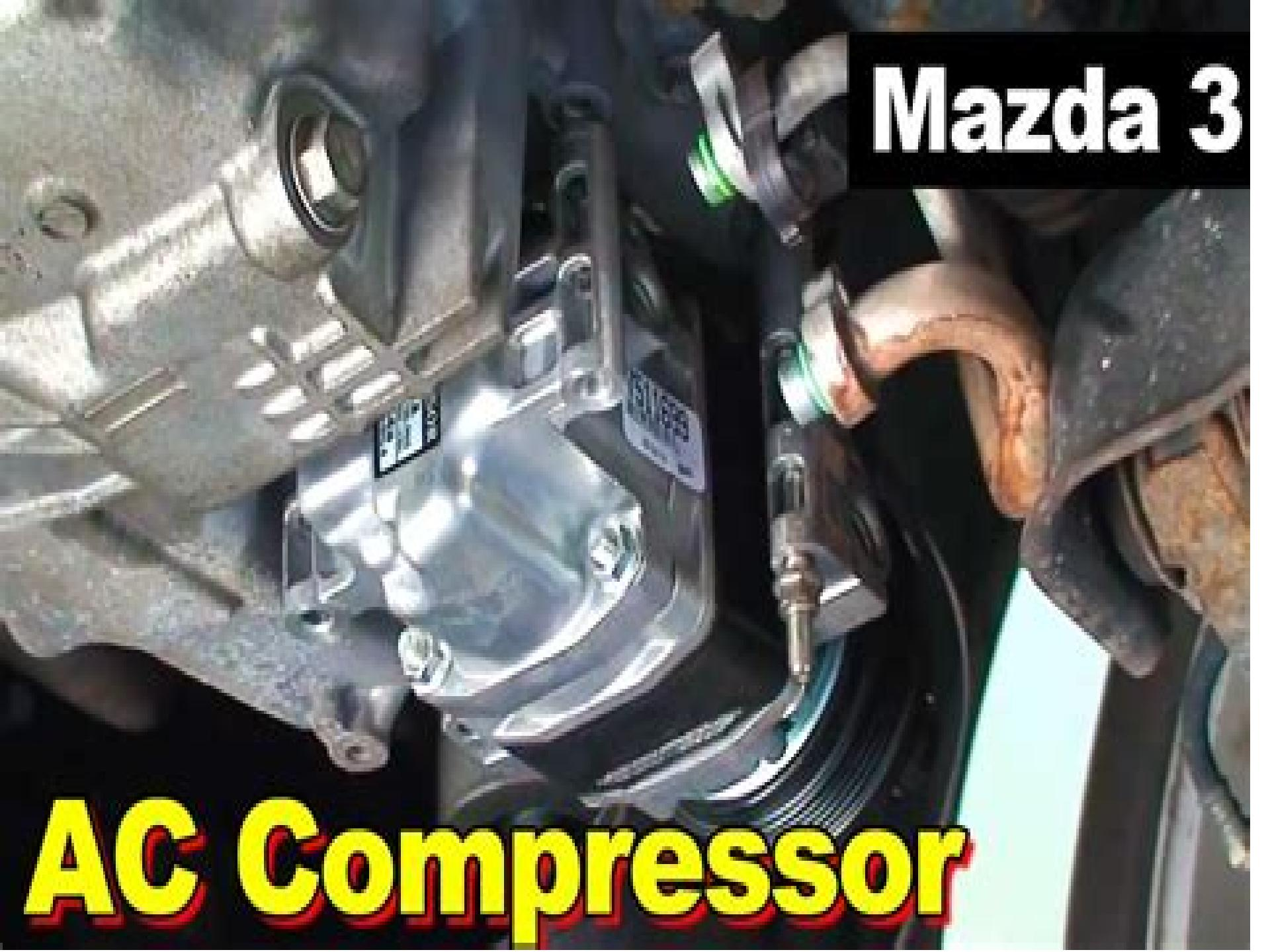
A close-up photograph of the AC compressor mounted on the front of a Mazda 3 engine. The compressor is a silver, cylindrical component with a ribbed belt and a black belt. It is secured to the engine block with several bolts. The background shows various engine components like hoses and a air cleaner. The lighting is bright, highlighting the metallic surfaces of the engine parts.
