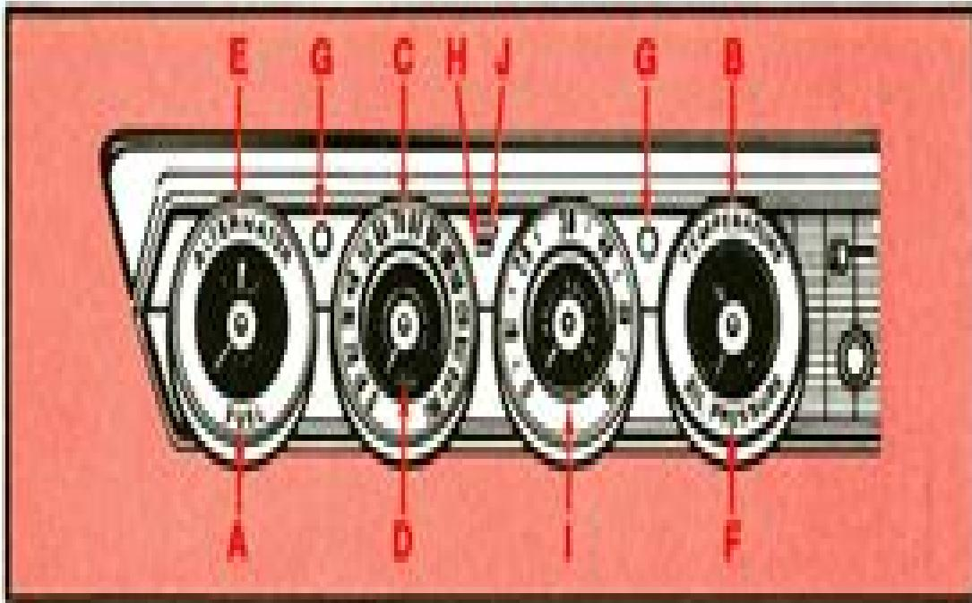
**E. ALTERNATOR INDICATOR**—Indicates whether battery is being charged or discharged. Pointer will normally stay centered when battery is fully charged and lights or accessories are not in use.
