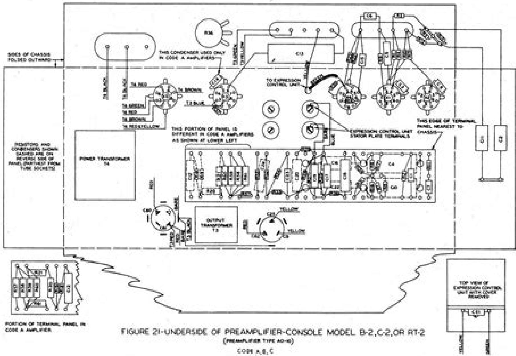
FIGURE 21-UNDERSIDE OF PREAMPLIFIER-CONSOLE MODEL B-2,C-2,OR RT-2
