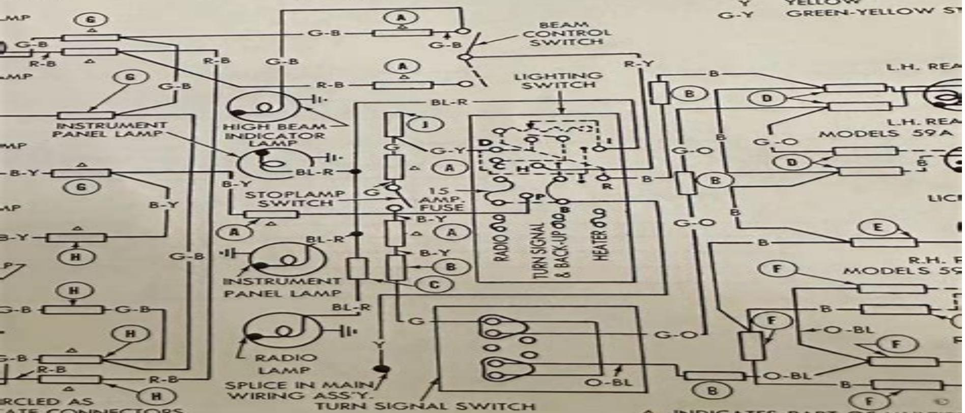
Exterior & Instrument Lamp Circuits.
