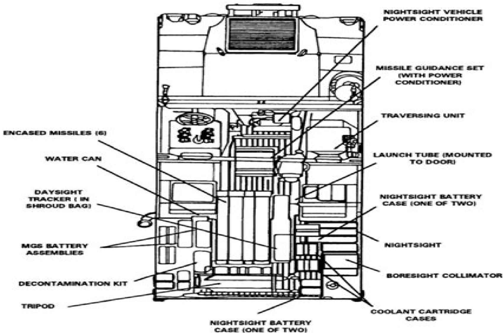
Figure 3-2. Stowing M220A1 on M966.
